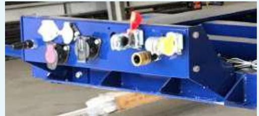
The couplings on the tractor should match the couplings of the trailer.
